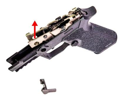
**4.** Pull up on the receiver rails, and then rotate the fire control assembly up.
