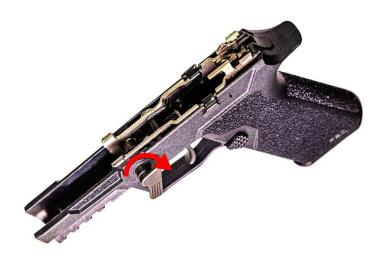
2. Remove the takedown lever (Turn and pull simultaneously).
