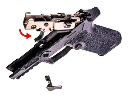
2. Press down on the receiver rails and pivot the fire control assembly into position.
