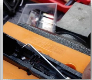
Use small tools or blast air to clean out pockets
