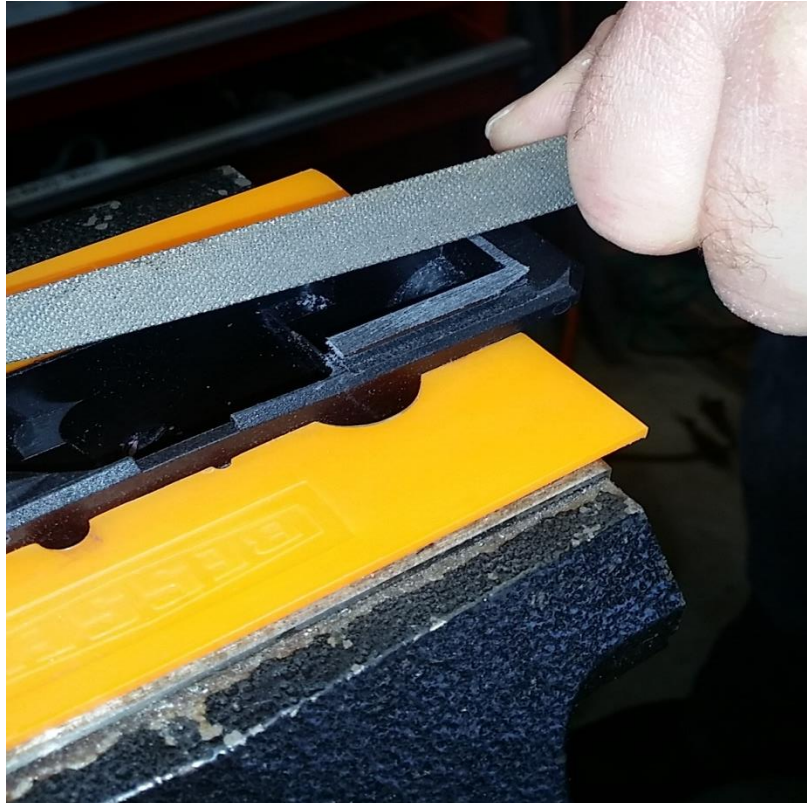
Example of a file being used to carefully bring down the material for custom fitment. Use 220 grit sand paper to finish
