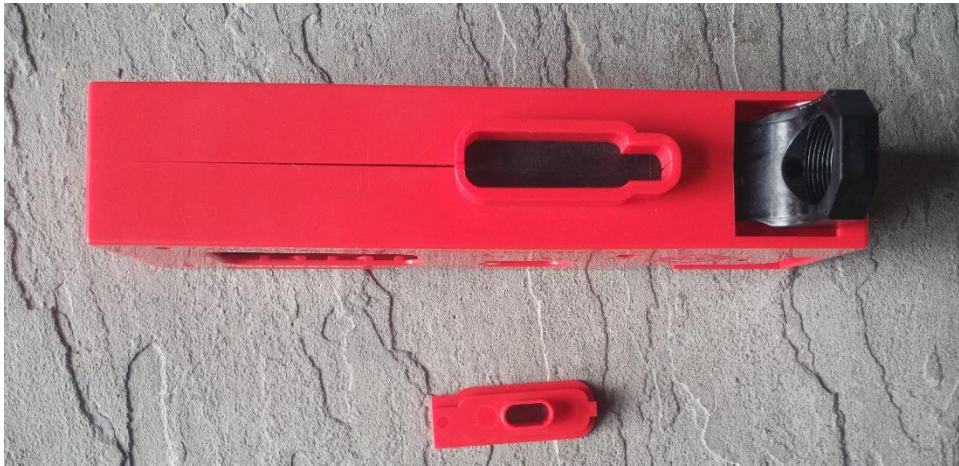
Top view with the Trigger Jig insert which snaps into the top of the jig
